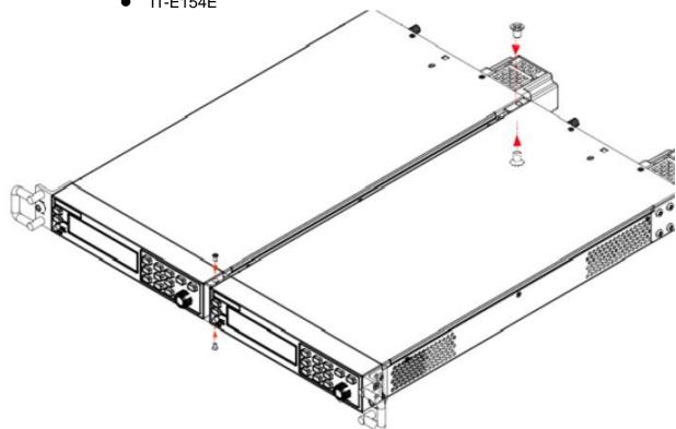
4. The user may install the two rack-mounted instruments on a standard cabinet. The size for rack-mounted instrument is as shown below. (Unit: mm)
