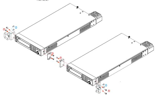
3. As shown below, combine two sets of instruments mounted with left and right racks. Use screws to fix the two sets of instruments from up to down.
